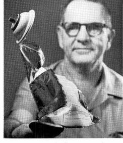
BOMB IN DISGUISE. This pressurized spray can suddenly became a lethal weapon after it inadvertently was placed on top of a transformer. Induction heating caused it to explode. The razor-edged and shattered can narrowly missed Sam Waldorf (4221).
